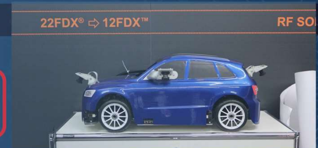
360° Surround View Demo Setup Demo-Car with 4 cameras
